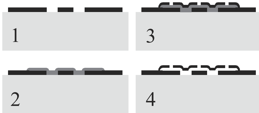
Figure 4.10: Outline of the fabrication process for the grounded-membrane sensor structure. In this case no attempt was made to obtain an extremely flat membrane.
