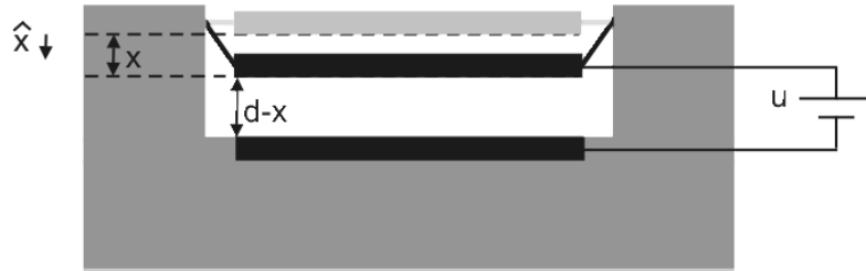
Figure 2.6: Schematic drawing of a parallel plate capacitor with one moveable plate.
